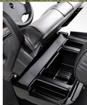
Front row under-seat storage tray with multiple compartments
